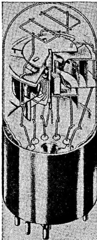
Figure 4-18. Cutaway view of the Phasitron tube, which is used as the modulator and upon which the operation of the GE f-m transmitter is based.
